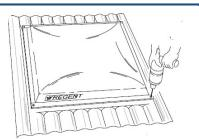
Raw edges of components of Regent Skylights & cut edges of roofing iron are sharp. Select location of "Corrolux" corrugated iron skylight on roof clear of obstruction, rafters & battens
