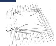
Fit Dome with trims supplied. Join corners of trim with one pop rivet at the intersection of each corner only.
