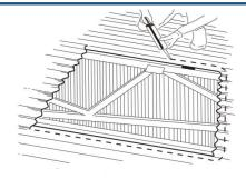
Place bead of silicone sealant along top of Skylight (ridge side) only, this will provide sealing between underside of roof & skylight as shown in step 7.
