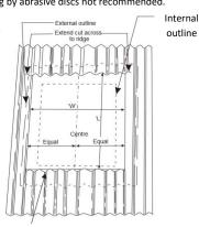
top lap to support roof Turn up bottom of corrugations on low end of cut
